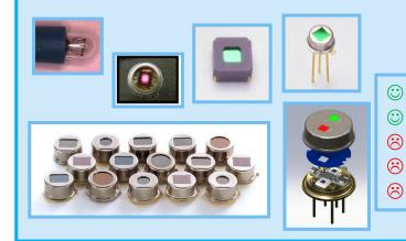
Many gases have IR absorptions due to molecular rotation & vibration Broadband source / interference filter selects required region of spectrum
