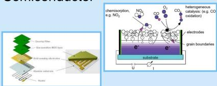
Porous semiconducting metal oxide Chemically adsorbed oxygen on surface - **[O]ads** Can react with many gases when heated (100-600°C) Change in **[O]ads** alters oxide electrical resistance No consumable element
