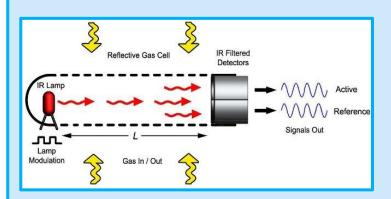
Sources and detectors – thermal or photonic Bulb, MEMs hotplate, LED Thermopile, pyroelectric, photodiode
