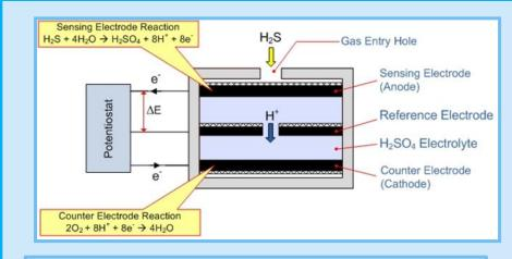
Electrodes – precious metal (Pt black) on PTFE tape Electrolytes – strong acid ( $H_2SO_4$ ) Wicks and separators - retain & transport electrolyte Target gas reaction - sensing electrode
